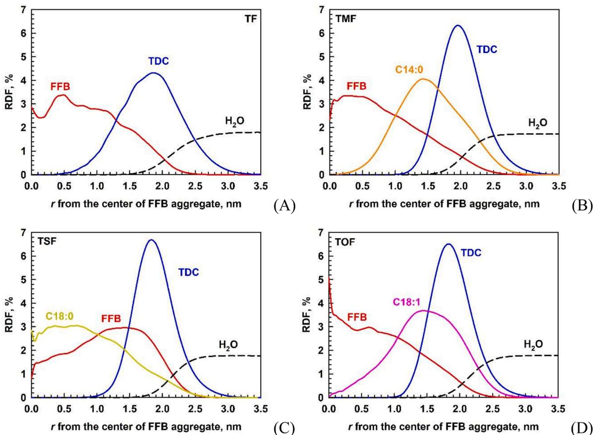
Fig. 5. Scaled RDFs calculated from the center of the FFB aggregates for each type of molecules in the systems: FFB - red, (A) TDC - blue, (B) C14:0 - orange, (C) C18:0 - yellow, and (D) C18:1 - pink; water - black dashed line.
