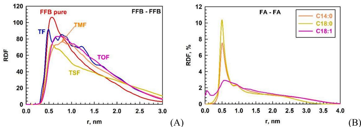
Fig. 4. RDF between the center of geometries of the (A) fenofibrate molecules and (B) fatty acids molecules in the systems without acids (red line), in the presence of TDC, TF (blue line), TDC + C14:0, TMF (orange line), TDC + C18:0, TSF (yellow line), TDC + C18:1, TOF (pink line).
