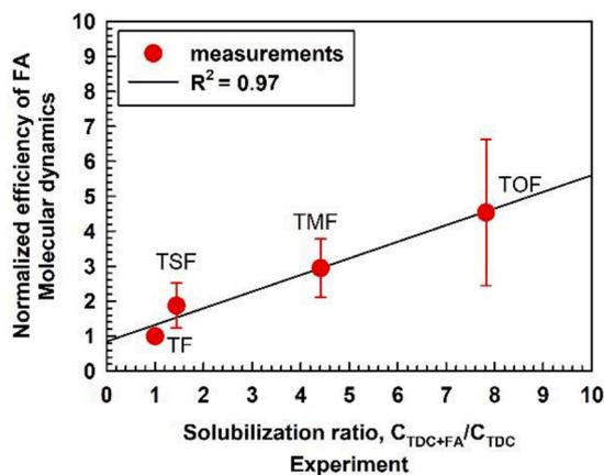
**Fig. 7.** Correlation plot between the calculated efficiency of the excipients in reducing the SASA of the FFB molecules and the experimentally measured solubilization ratio. Averages and standard deviations from two independent trajectories are shown.
