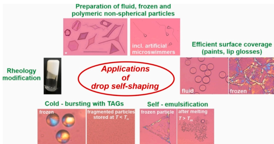
Fig. 30. Examples illustrating possible applications of the studied phenomena. These include – preparation of particles with non-spherical shapes, including artificial microswimmers; spontaneous drop size decrease without mechanical energy input via the cold-bursting and self-emulsification processes; emulsion rheology modification while the continuous phase is still in liquid state, etc. *Note that this is not a directly obtained microscopy image, but is a collage with real deformed particles, combined together (all other images included in the paper are as directly observed in the experiments).
