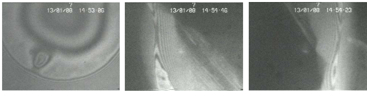
Fig. A.3. HFBII-stabilized emulsion films with fresh oil/water interfaces: (a–c) evolution of a o/w/o film from aqueous solution with 10^{-3} wt % HFBII – fast transition to S-bilayer, which is stable. Photos for aged interfaces are not shown, because there was no difference with fresh interfaces. The horizontal length of each photo corresponds to 300 \mu\text{m} .
