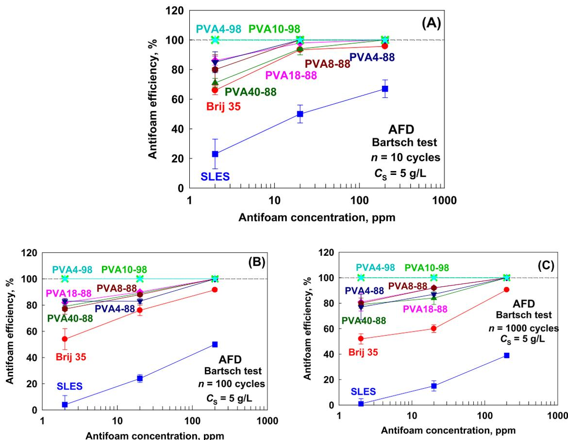
Fig. 1. Antifoam efficiency,  $AE$ , to destroy the foam generated after (A) 10; (B) 100 and (C) 1000 shaking cycles in Bartsch test from 5 g/L solutions of SLES (blue squares); Brij 35 (red circles); PVA 40–88 (green triangles up); PVA 18–88 (pink diamonds); PVA 8–88 (brown hexagons); PVA 4–88 (blue triangles down); PVA 10–98 (green stars) and PVA 4–98 (cyan X) at different antifoam concentrations in which the antifoam is dosed as antifoam dispersion.
