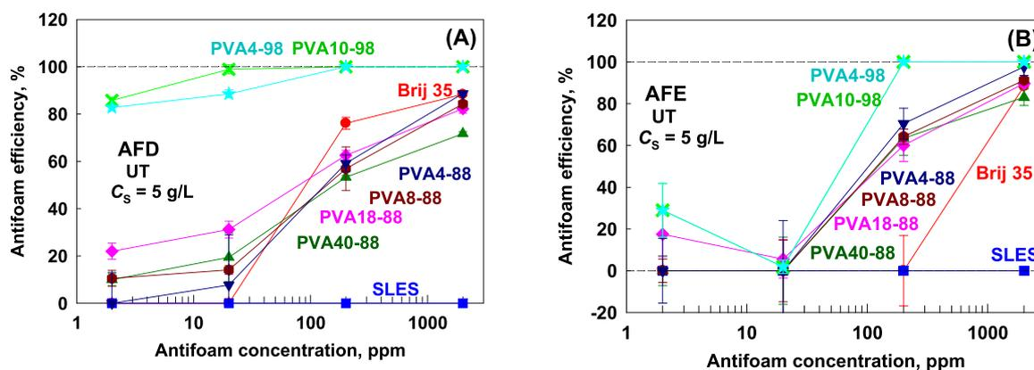
Fig. 5. Antifoam efficiency,  $AE$ , to destroy the foam generated in UT from 5 g/L solutions of SLES (blue squares); Brij 35 (red circles); PVA 40-88 (green triangles up); PVA 18-88 (pink diamonds); PVA 8-88 (brown hexagons); PVA 4-88 (blue triangles down); PVA 10-98 (green stars) and PVA 4-98 (cyan X) for antifoam added as (A) antifoam dispersion and (B) antifoam emulsion.
