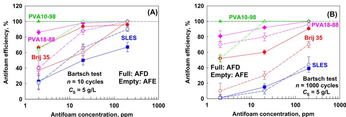
Fig. 2. Antifoam efficiency,  $AE$ , as a function of antifoam concentration,  $C_{AF}$ , after (A) 10 and (B) 1000 cycles in Bartsch test for antifoam dosed as AFE (empty points) and AFD (full points) in 5 g/L solution of SLES (blue squares); Brij 35 (red circles); PVA 18–88 (pink diamonds); PVA 10–98 (green triangles).
