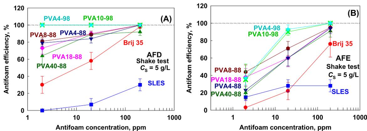
Fig. 4. Antifoam efficiency,  $AE$ , to destroy the foam generated in shake test from 5 g/L solutions of SLES (blue squares); Brij 35 (red circles); PVA 40–88 (green triangles up); PVA 18–88 (pink diamonds); PVA 8–88 (brown hexagons); PVA 4–88 (blue triangles down); PVA 10–98 (green stars) and PVA 4–98 (cyan X) for antifoam added as (A) antifoam dispersion and (B) antifoam emulsion.
