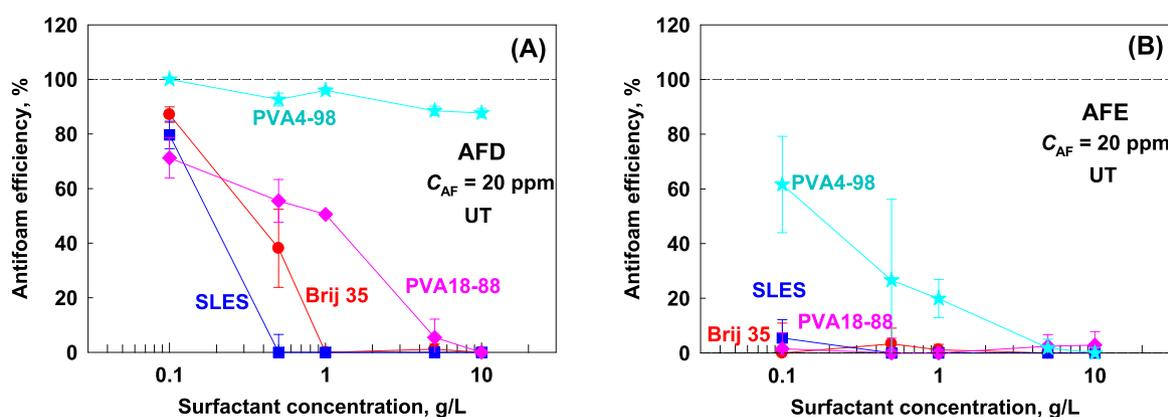
Fig. 6. Antifoam efficiency,  $AE$ , as a function of surfactant concentration for foams formed in UT from SLES (blue squares); Brij 35 (red circles); PVA 18-88 (pink diamonds); PVA 4-98 (cyan stars) solutions in presence of 20 ppm AF introduced as (A) antifoam dispersion and (B) antifoam emulsion.
