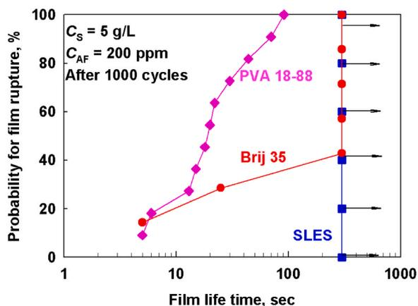
**Fig. 10.** Probability for film rupture after certain period of time for films formed in capillary cell from 5 g/L PVA 18–88 (pink diamonds); Brij 35 (red circles); SLES (blue squares) solutions containing 200 ppm AF, dosed as AFD, which have been shaken 1000 cycles in Bartsch test. The arrows show that the film life time is longer than 300 s, which is the longest time during which the films were observed.
