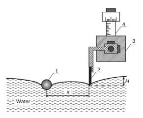
**FIGURE 7.25** Experimental setup for studying the capillary interaction between a floating particle (1) and a vertical hydrophobic plate (2) separated at a distance, *x*. The edge of the plate is at a distance, *H*, lower than the level of the horizontal liquid surface far from the plate; (3) and (4) are micrometric table and screw [311,312].
