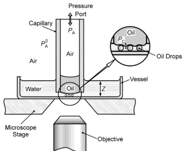
**Figure 3.** Basic scheme of the film trapping apparatus. Scheme of the droplets trapped between the oil-water interface and the substrate (see the magnification lens).
