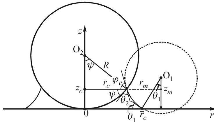
Fig. 11.3. In toroid approximation the generatrix of the profile of the capillary bridge is approximated with a circle (with center at  $O_2$  in the figure).  $\theta_1$  and  $\theta_2$  are the three-phase contact angles at the surfaces of the solid plate and the spherical particle of radius  $R$ , respectively.
