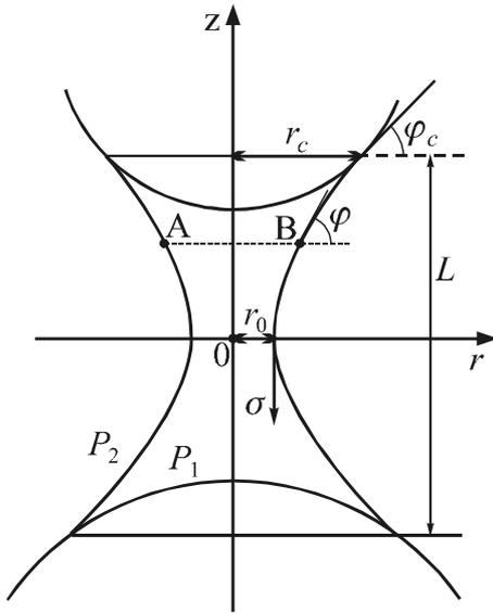
Fig. 11.2. Sketch of the capillary bridge between two axisymmetric particles or bodies.  $P_1$  and  $P_2$  are the pressures inside and outside the bridge of length  $L$ ;  $r_0$  and  $r_c$  are the radii of the neck and the contact line;  $\varphi_c$  and  $\varphi$  are the values of the meniscus slope angle at the contact line and at an arbitrarily chosen section  $AB$ .
