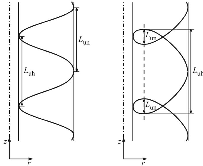
Fig. 11.5. Geometrical upper limits for the stability of capillary bridges: (a) distances between two closest points with vertical tangents for an unduloid with “neck”,  $L_{un}$ , and with “haunch”,  $L_{uh}$ ; (b) distances between two closest points with horizontal tangents for a nodoid with “neck”,  $L_{un}$ , and with “haunch”,  $L_{uh}$ .
