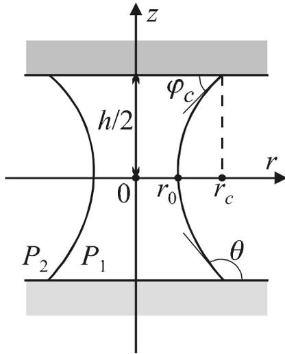
Fig. 11.4. Capillary bridge formed between two plane-parallel solid surfaces separated at a distance  $h$ ;  $r_0$  and  $r_c$  are the radii of the neck and the contact line;  $\varphi_c$  is the contact angle measured across the phase of the bridge.
