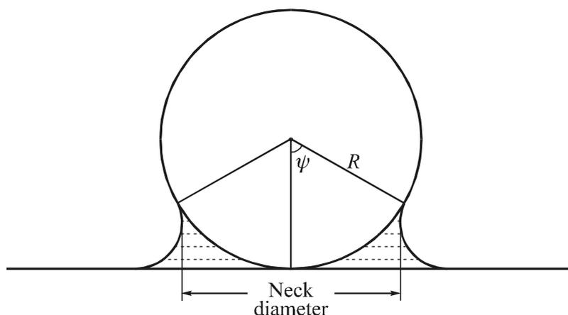
Fig. 11.1. Liquid bridge between a spherical particle and a planar solid surface.
