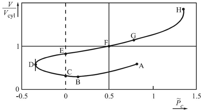
Fig. 11.6. Plot of the volume of a liquid bridge,  $V$ , scaled with the volume of the cylindrical bridge,  $V_{cyl}$ , against the dimensionless pressure difference across the meniscus surface,  $\tilde{P}_c$ , see Eq. (11.64); the bridge is symmetric like that in Fig. 11.4;  $V$  and  $\tilde{P}_c$  vary at fixed contact line radius  $r_c$  and fixed length  $L$  of the bridge {after Ref. [60]}.
