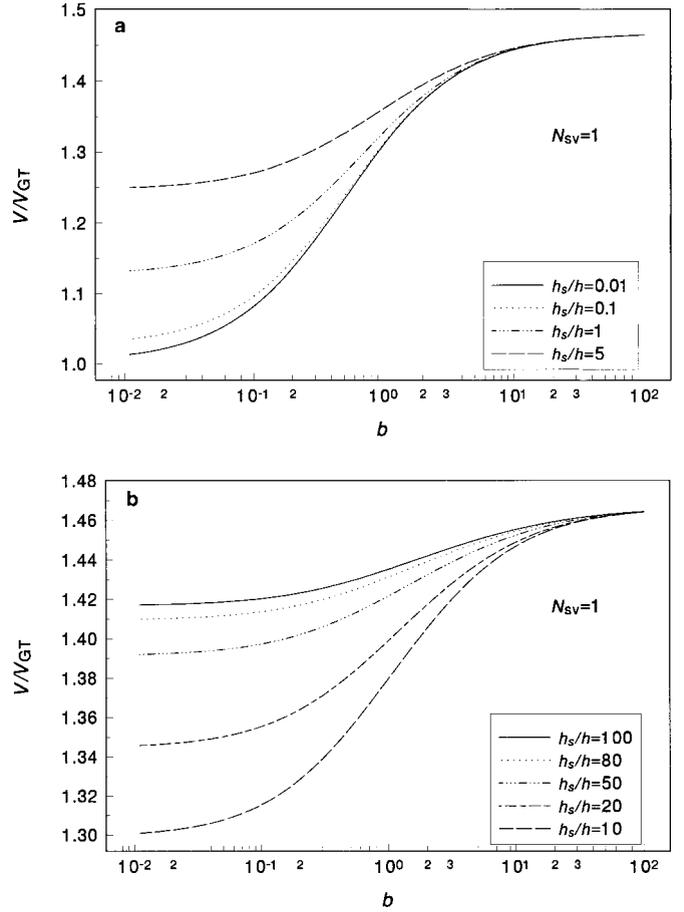
**FIG. 5.** Dimensionless approaching velocity,  $V/V_{GT}$ , as a function of the bulk diffusion parameter  $b$ : (a) for  $N_{sv} = 1$  and low and moderate surface diffusivities; (b) for  $N_{sv} = 1$  and high surface diffusivity.
