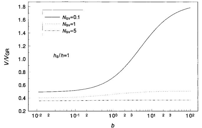
**FIG. 8.** Dimensionless velocity of film thinning,  $V/V_{GR}$ , as a function of the bulk diffusion parameter  $b$  for  $h_s/h = 1$ ,  $N_{rf} = 1$  and different values of surface diffusion number,  $N_{sv}$ .
