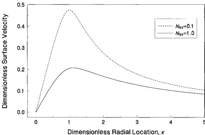
**FIG. 6.** Dimensionless surface velocity,  $\tilde{U}$ , distribution at a given distance  $x$  for  $b = 1$ ,  $h_s/h = 1$ ,  $N_{rf} = 1$  and different values of the parameter  $N_{sv}$ .
