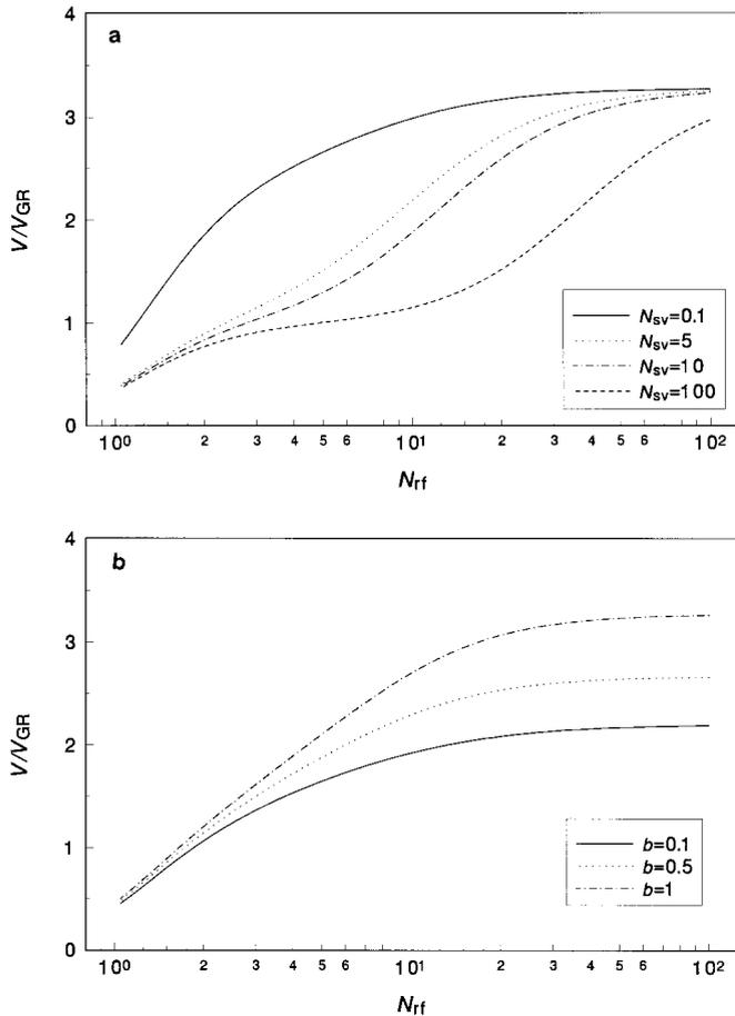
**FIG. 9.** Variation of the mobility factor,  $V/V_{GR}$ , with the dimensionless film radius,  $N_{rf}$ : (a)  $b = 1$ ,  $h_s/h = 1$  and different surface viscosities; (b)  $N_{sv} = 1$ ,  $h_s/h = 1$  and different bulk diffusivities.
