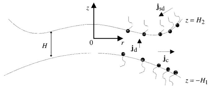
**FIG. 2.** Schematic picture of a thin liquid film between two deformed bubbles. The cylindrical coordinate system is  $Orz$ . The surfactant bulk and surface diffusion fluxes are respectively  $\mathbf{j}_d$  and  $\mathbf{j}_{sd}$ . The convection surfactant flux at the interface is  $\mathbf{j}_c$ .
