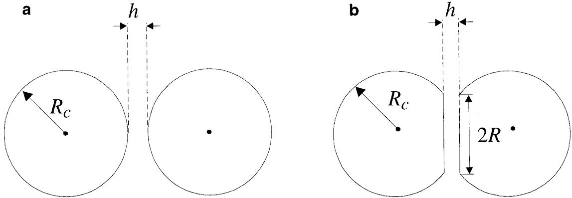
**FIG. 1.** Sketch of two bubbles of radius  $R_c$  separated at a surface-to-surface distance  $h$ . (a) For large  $h$  the bubbles are spherical; (b) for small  $h$  the bubbles are deformed and a plane-parallel film with radius  $R$  surrounded by a meniscus appears.
