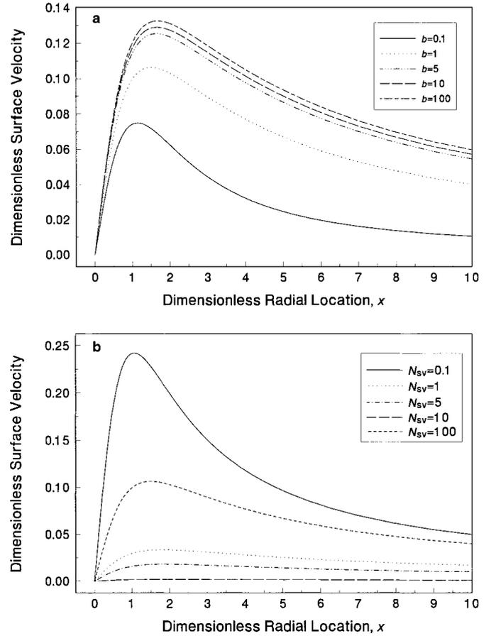
**FIG. 3.** Dimensionless surface velocity,  $\tilde{U}$ , distribution at a given distance  $h$ : (a) for  $N_{sv} = 1$ ,  $h_s/h = 1$ , and different values of the parameter  $b$ ; (b) for  $b = 1$ ,  $h_s/h = 1$ , and different values of the parameter  $N_{sv}$ .
