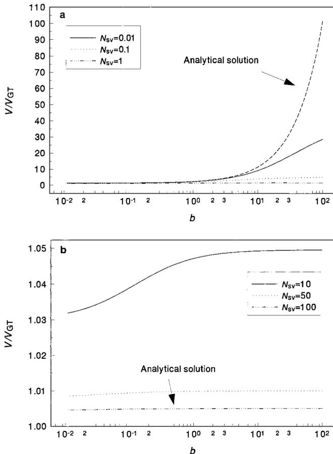
**FIG. 4.** Variation of the mobility factor,  $V/V_{GT}$ , with the bulk diffusion parameter  $b$ : (a) for  $h_s/h = 1$  and low and moderate values of the parameter  $N_{sv}$ ; (b) for  $h_s/h = 1$  and high values of the parameter  $N_{sv}$ .
