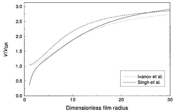
**FIG. 10.** Comparison of the mobility factor  $V/V_{GR}$  as predicted by Ivanov *et al.* (12) and Singh *et al.* (3) for finite plane-parallel film and our model. The parameters in the calculations are  $b = 1$ ,  $h_s/h = 1$  and  $N_{sv} = 10$ .
