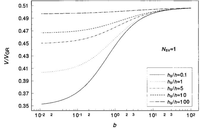
**FIG. 7.** Variation of the mobility factor,  $V/V_{GR}$ , with the bulk diffusion parameter  $b$  for  $N_{sv} = 1$ ,  $N_{rf} = 1$  and different values of  $h_s/h$ .
