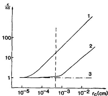
FIG. 1. Comparison of the values of the line tension  $\kappa_a$ , calculated from the approximated Eqs. [2] (curves 1 and 2) and [3] (curve 3), with  $\kappa$  calculated from the general Eq. [1] for different  $r_c$ . Curves 1 and 3 are with the values of  $\Pi_2$ ,  $t_1$ , and  $a$  from (6), and curve 2 is with the respective values from (5).
