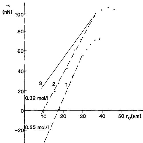
FIG. 2. Our data from (2) for  $\kappa$  vs  $r_c$  at two different electrolyte concentrations (curves 1 and 2). Curve 3 is calculated from Eq. [4] with  $N = \frac{5}{8}$  and values of  $\Pi_2$ ,  $t_1$  and  $a$  from Ref. (6).
