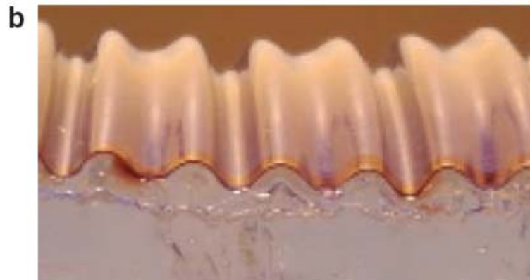
Polyester film (10 \mu\text{m} ) on gel substrate
